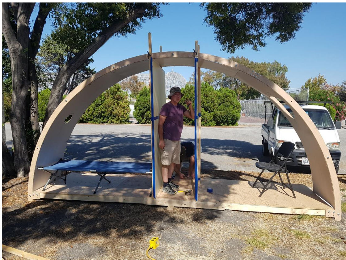
Structural mockup of a segment of the upper deck of the Mars Oz habitat module with the designer Willson at NASA Ames Research Center. Mars Society Australia image.
