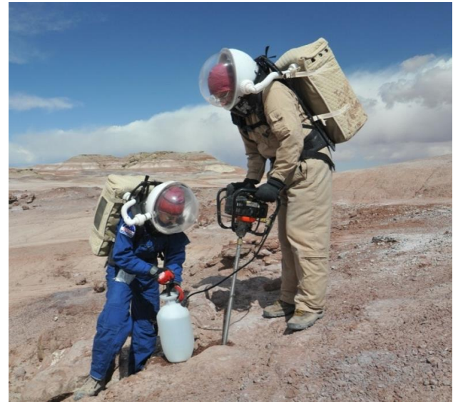
Carol Stoker (left) and author (right) using the Backpack drill near MDRS for full sim drilling. Mars society photo.
